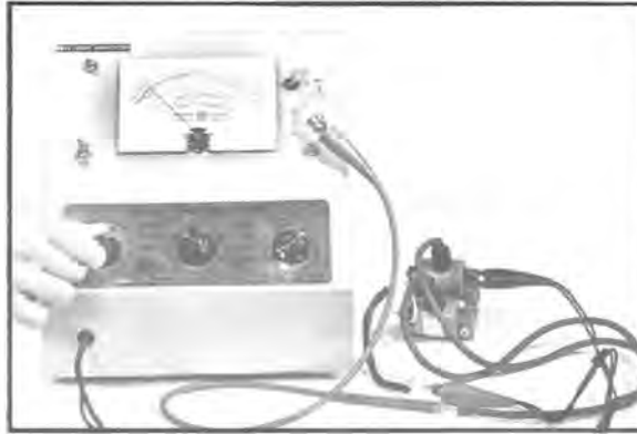
Test No. 5 — Gap Index Test (Do not make this test on a metal bench)
