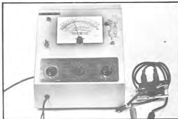
Test No. 1 – Secondary Continuity
