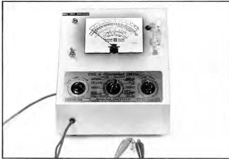
Test No. 3 — Condenser Leakage
