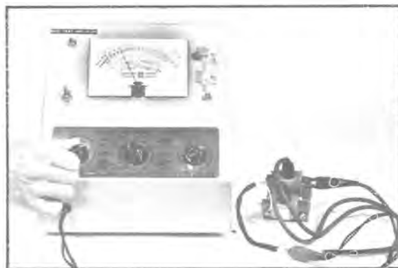
Test No. 4 — Minimum Coil Firing Test (Do not make this test on a metal bench)
