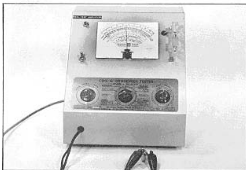
Test No. 1 — Condenser Capacity
