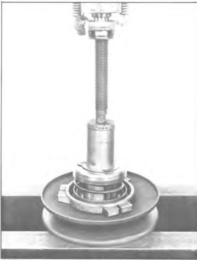
Fig. 73 — Pressing Pulley So That Locking Nuts Can Be Removed
