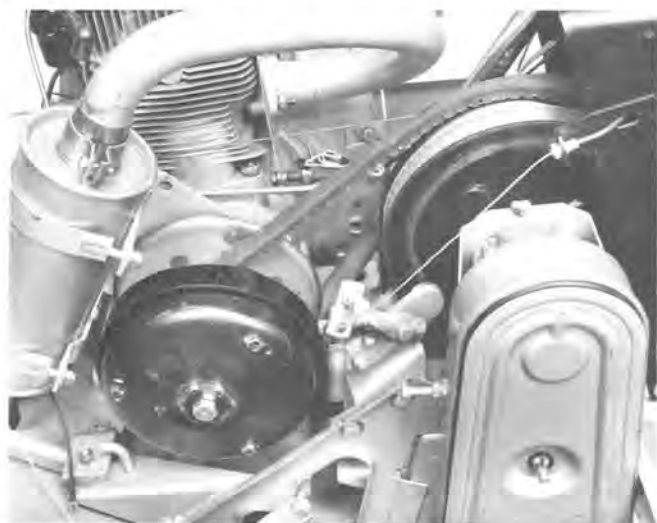
Fig. 8 — Removing Drive Belt from Driven Pulley (L 380 Engine Pulley Arrangement Shown)
