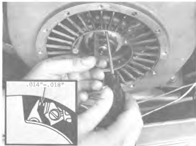
Fig. 18 — Checking Breaker Point Gap
