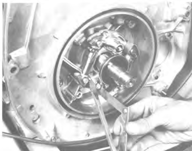
Fig. 39 — Setting Breaker Point Gap
