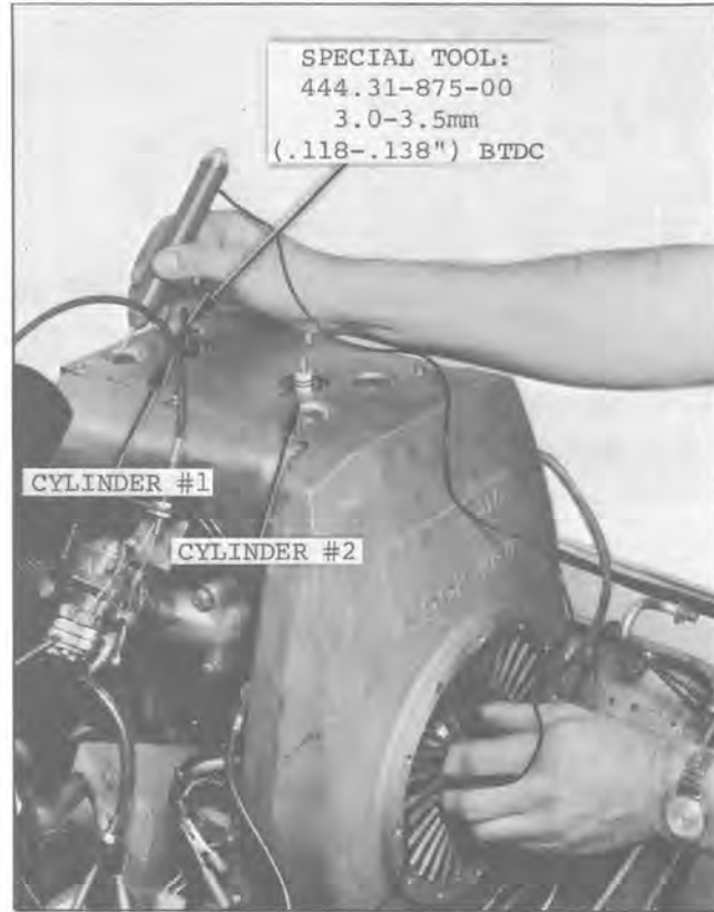
Fig. 25 — Timing Engine (W/Timing Gauge)
