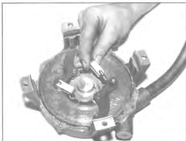
Fig. 31 — Installing Brake Spring Compressing Tools
