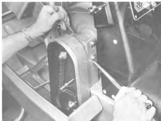
Fig. 16 — Adjusting Chain Tension
