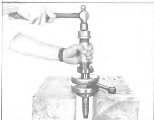
Fig. 30 — Tapping Heated Bearing Onto Crankshaft
