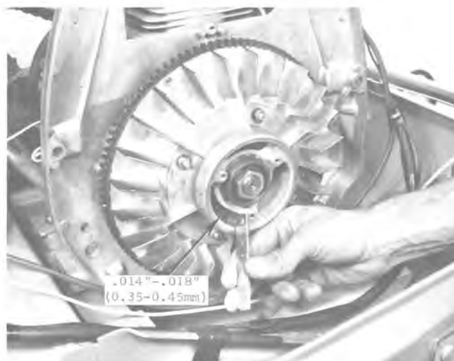
Fig. 34 — Checking Breaker Point Gap
