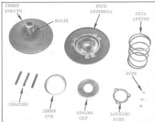
Fig. 74 — Driven Pulley Identification of Parts — L 297 Engine
