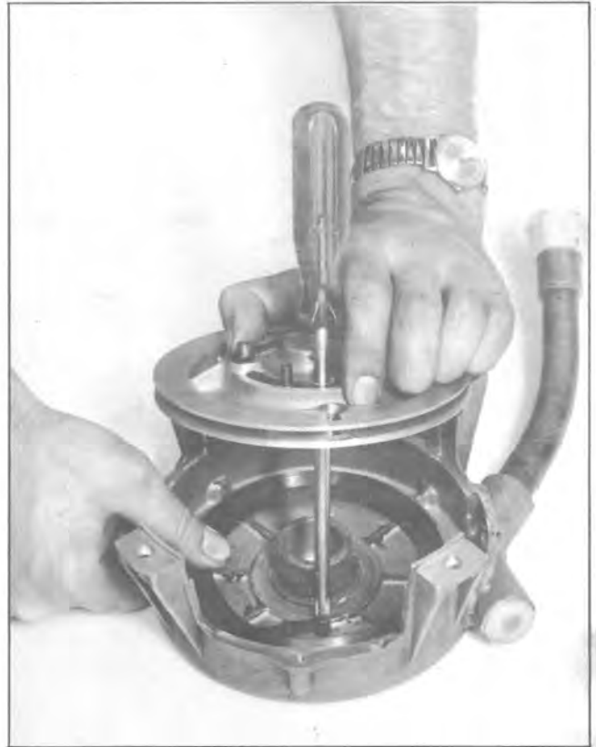
Fig. 29 — Removing Drum from Starter Housing
