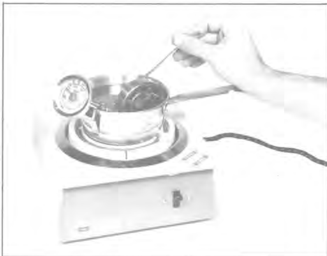
Fig. 29 — Heating Crankshaft Bearing Prior to Installation
