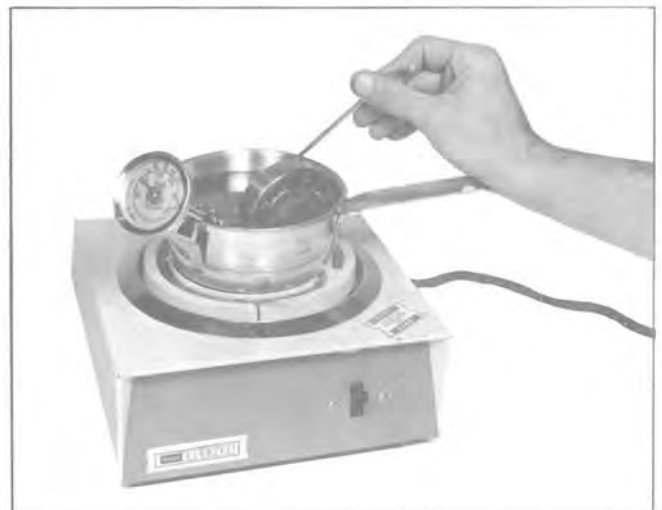
Fig. 14 — Heating Crankshaft Bearings Prior to Installation
