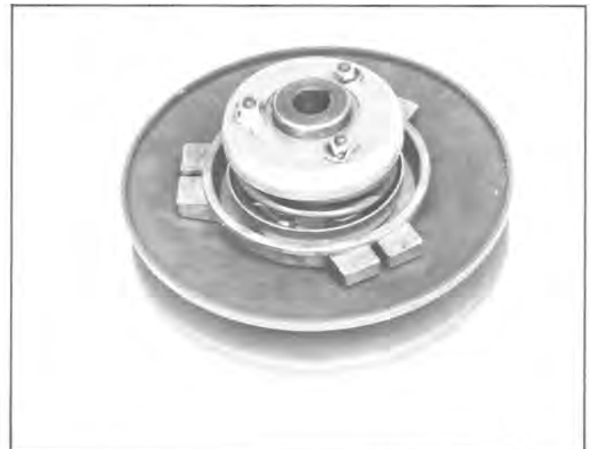
Fig. 72 — Driven Pulley Assembly Used with L 297 Engine
