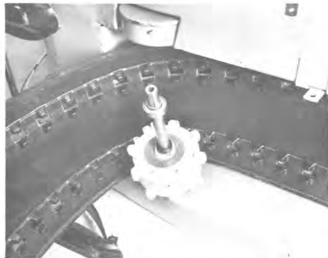
Fig. 84 — Axle Shaft Freed From Left-Hand Bearing
