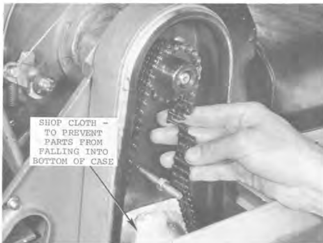
Fig. 15 — Removing Chain and Upper Sprocket
