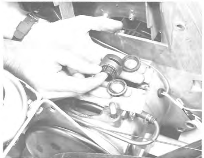
Fig. 18 — Removing / Installing Piston Pin Bearing and Retainers
