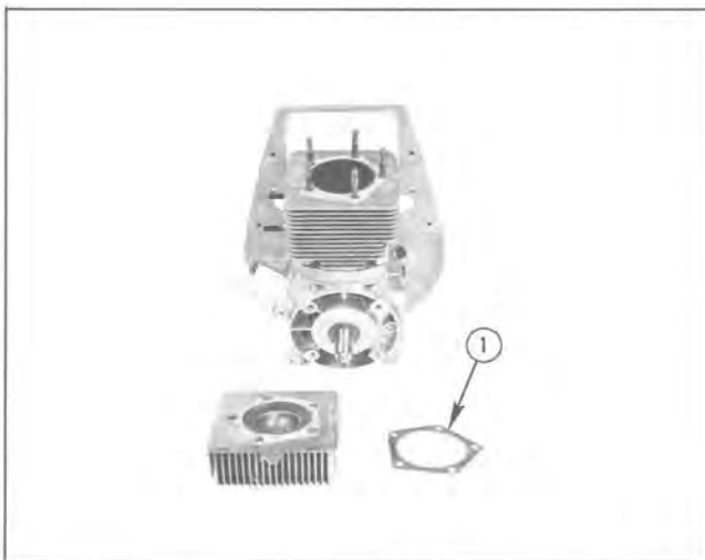
Fig. 12 — Cylinder Head &amp; Gasket On L 297 Engine
