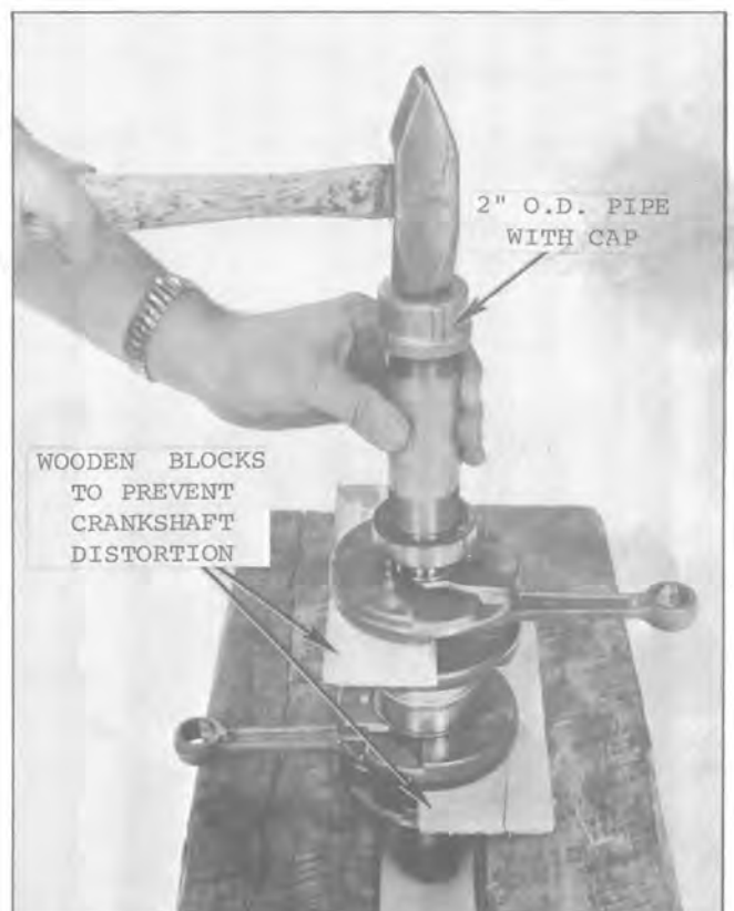
Fig. 15 — Installing Crankshaft Bearings
