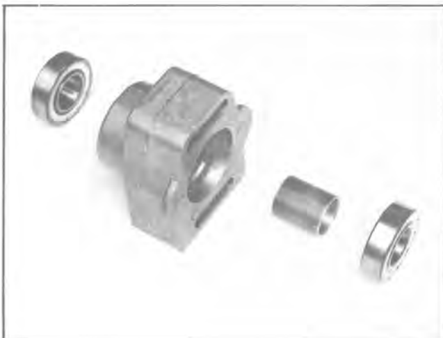
Fig. 12 — Bearing Block Disassembled
