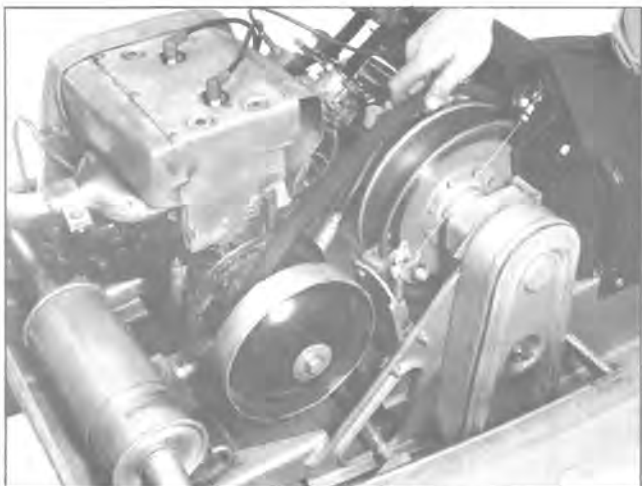
Fig. 2 — Removing/Installing Drive Belt
