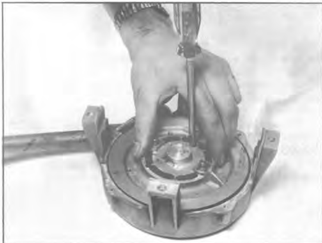
Fig. 28 — Disengaging Recoil Spring from Drum
