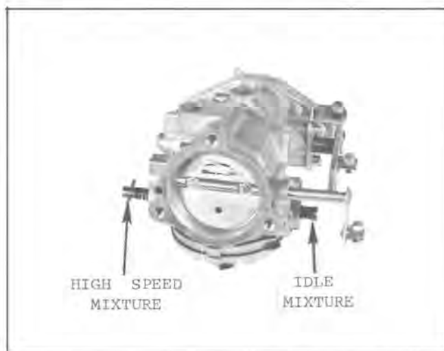
Fig. 48 — Model "HD" Carburetor Used with L 380 Engine
