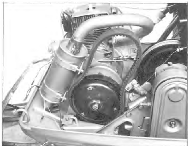
Fig. 9 — Removing Drive Belt from Drive Pulley (L 380 Engine Pulley Arrangement Shown)
