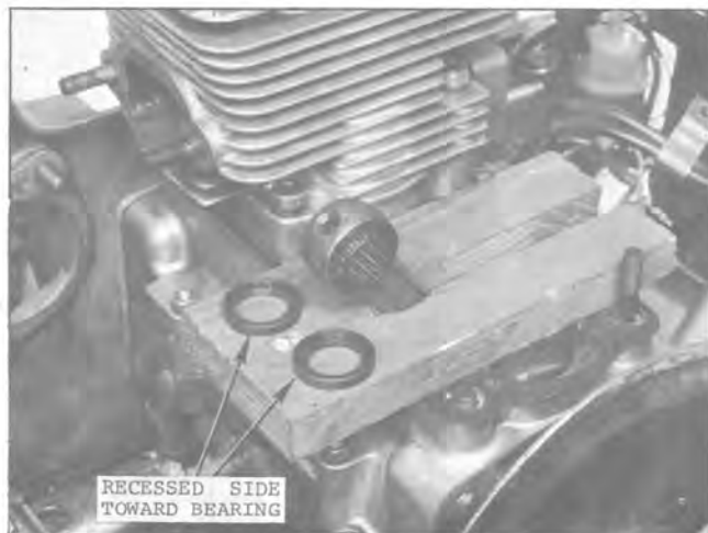
Fig. 8 — Piston Pin Bearing and Retainers
