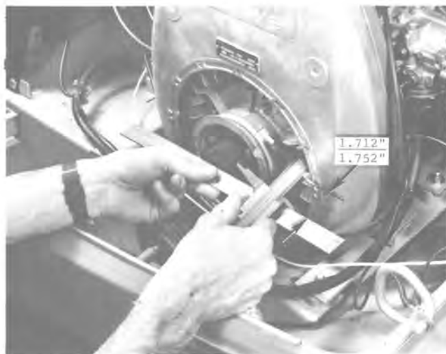
Fig. 42 — Checking Starter Carrier Adjustment
