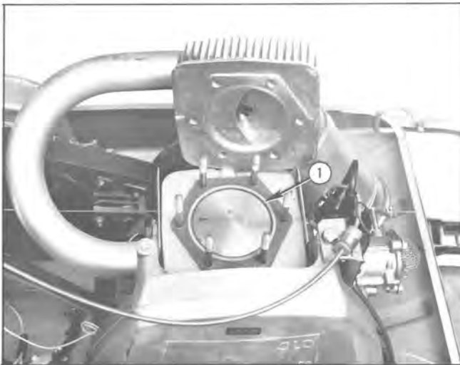
Fig. 11 — Cylinder Head &amp; Gasket On L 380 Engine
