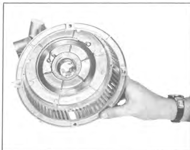
Fig. 45 — Starter Housing with Recoil Spring Installed
