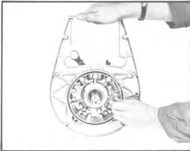
Fig. 24 — Removing / Installing the Crankcase Assembly Screws (L 297 Engine Shown)
