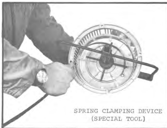
Fig. 46 — Replacing Recoil Spring
