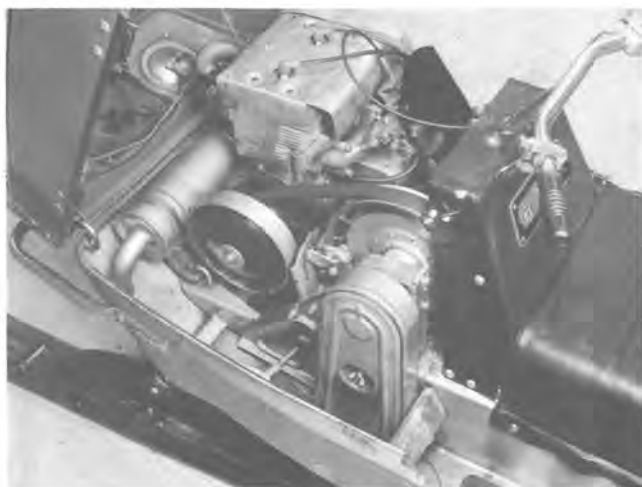
Fig. 1 — Engine and Drive Assembly Installed
