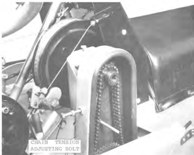
Fig. 66 — Removing Shaft From Upper Sprocket
