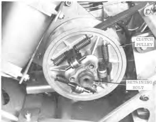
Fig. 54 — Drive Pulley Used with L 297 Engine (Cover Removed to Show Internal Parts)
