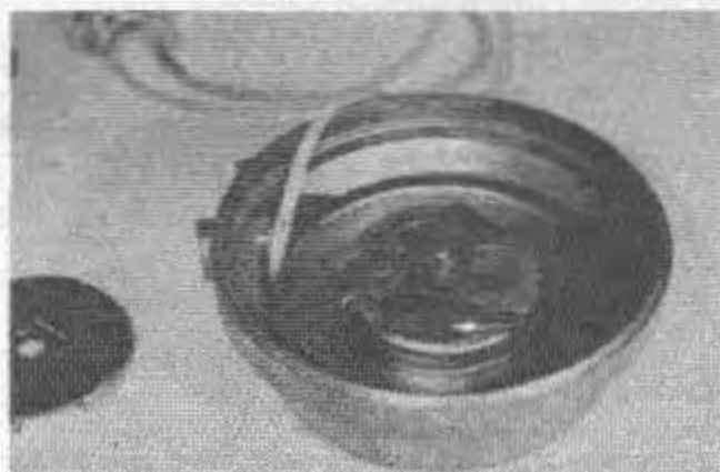
Fig. 35 — Pulley Cup Washer and Spring Installed
