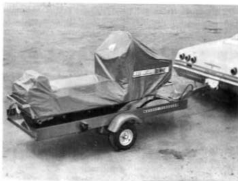
Fig. 21 - Transport Trailer and Protective Cover
