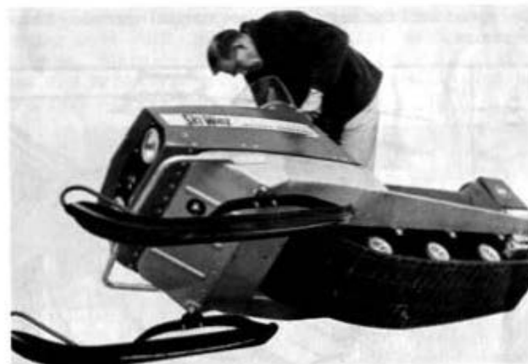
Fig. 2 - Breaking Machine Loose from Ice
