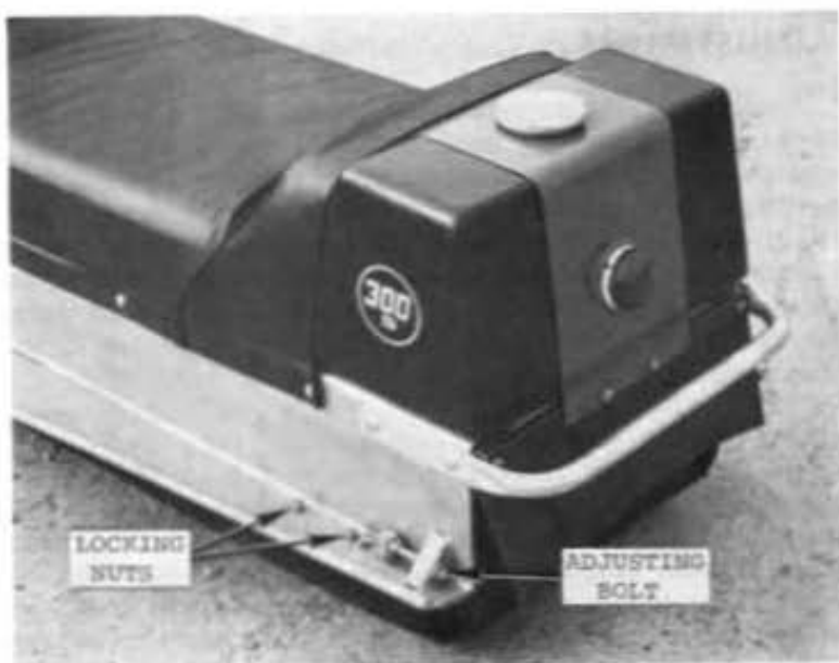
Fig. 4 - Track Tension Adjustment
