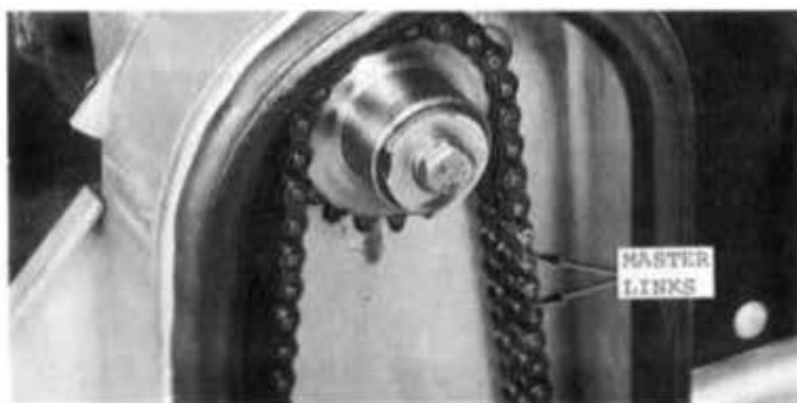
Fig. 14 - Drive Chain Replacement
