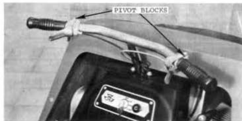
Fig. 8 - Throttle and Brake Control Adjustment
