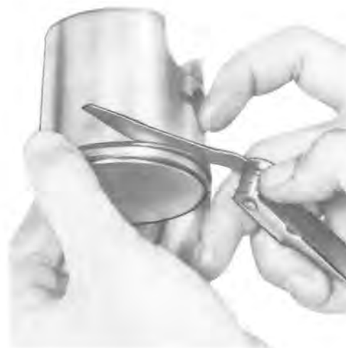
PISTON RING/GROOVE CLEARANCE TOP AND BOTTOM
