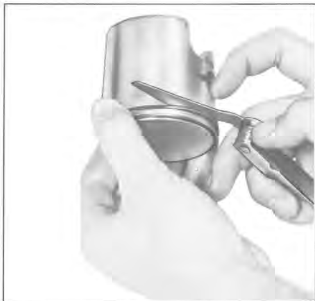
TOP RING/GROOVE CLEARANCE
