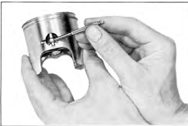
PISTON PIN BORE DIAMETER
