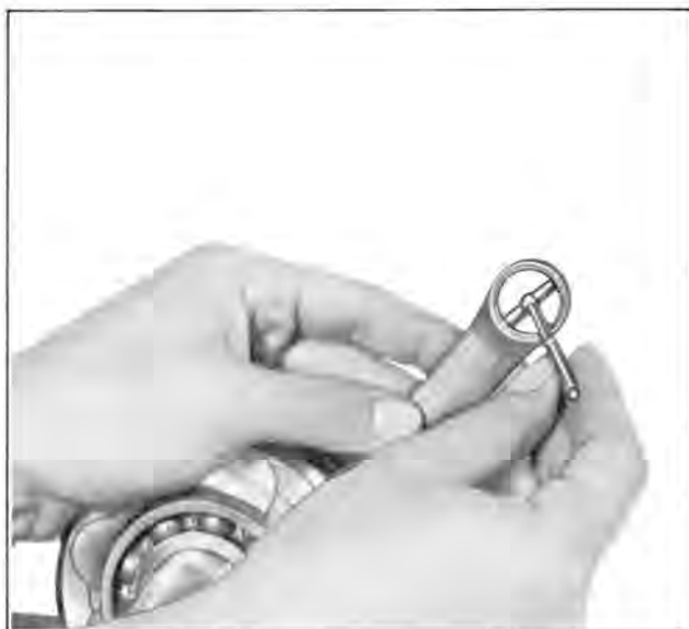
CONNECTING ROD SMALL END DIAMETER
