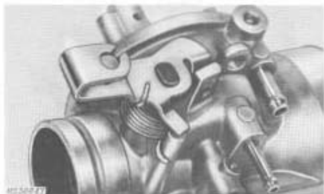
Fig. 17—Installing Throttle Lever and Spring
