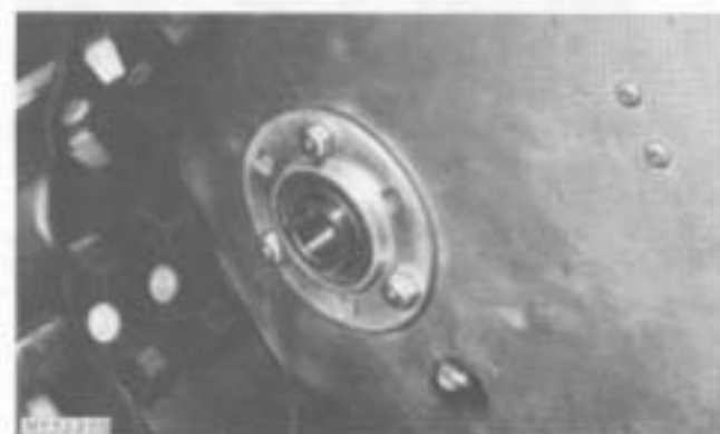
Fig. 6-Left-Hand Bearing Assembly Installed
