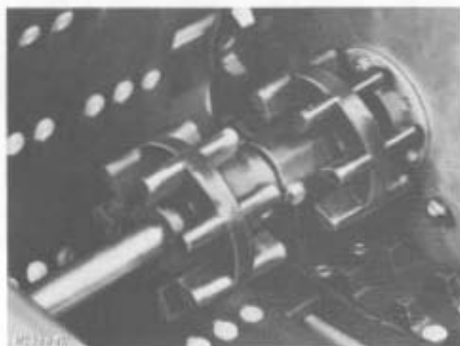
Fig. 7-Drive Shaft Installed in Left-Hand Bearing
