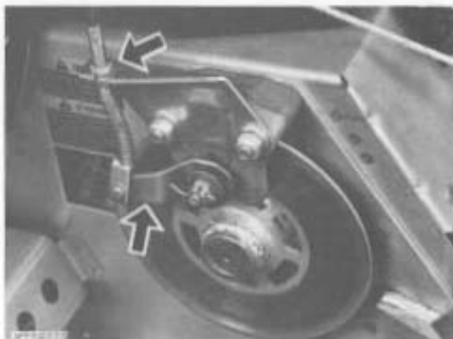
Fig. 6-Adjusting Brake Cable and Cam
