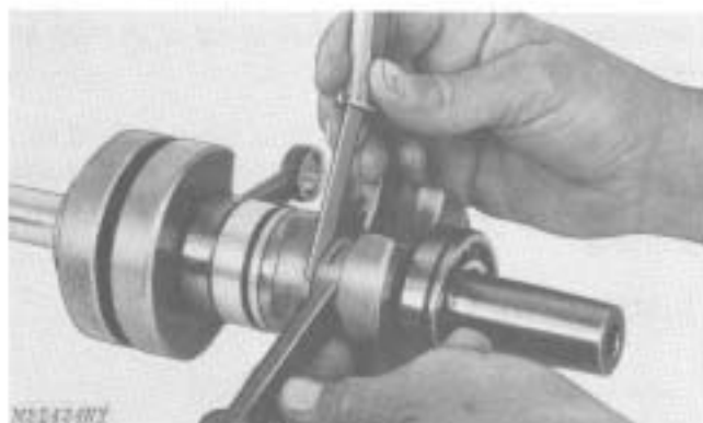
Fig. 16-Checking Connecting Rod Side Clearance
