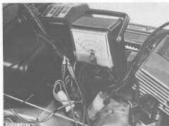
Fig. 5-Testing Engine Kill Switch
