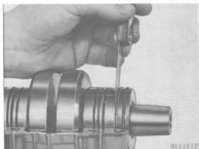
Fig. 33-Checking Crankshaft End Play
