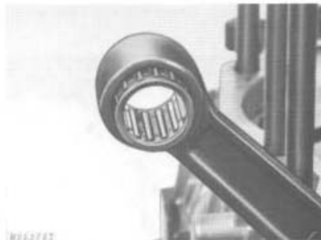
Fig. 16-Removing Piston Pin Needle Bearing
