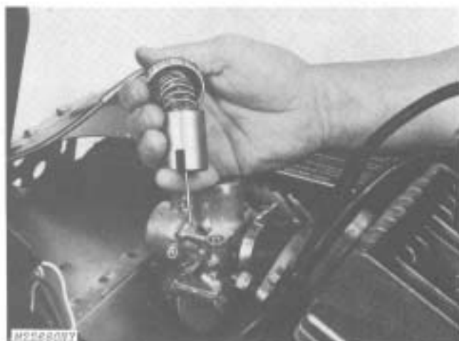
Fig. 2-Removing Throttle Valve Assembly
