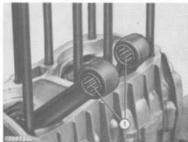
Fig. 35-Installing Piston Pin Needle Bearings
