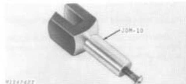
Fig. 4-Dial Indicator Mounting Bracket
