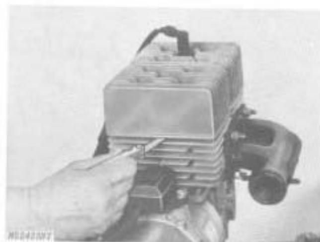
Fig. 14-Checking Cylinder For Distortion
