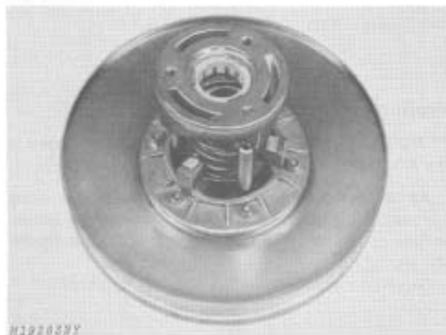
Fig. 14-Installing Cam With Spring
