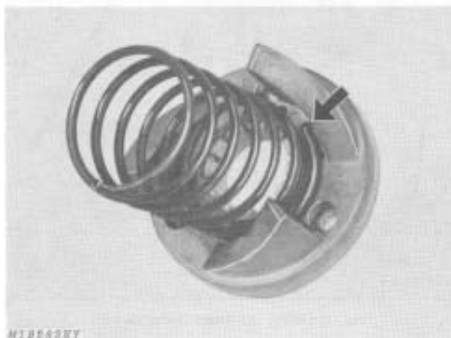
Fig. 13-Spring Installed in Cam
