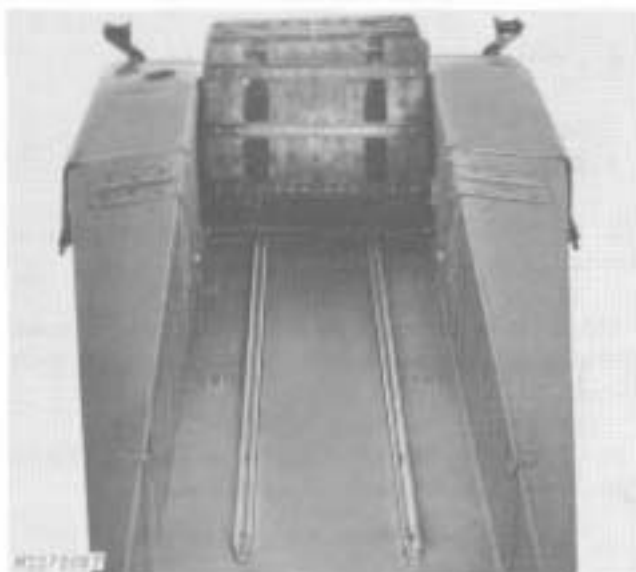
Fig. 5-Replacing Tunnel Wear Bars
