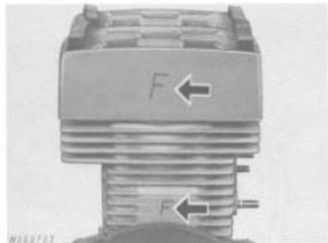
Fig. 13-Removing Cylinders and Heads
