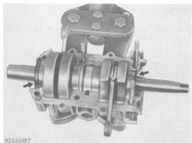
Fig. 20-Crankshaft Installed for Checking End Play
