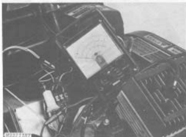
Fig. 2-Testing Alternator With Ohmmeter
