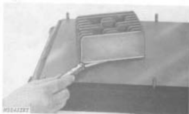
Fig. 13-Checking Cylinder Head For Flatness
