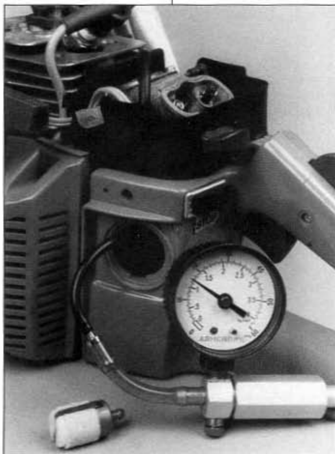
Pressure testing the fuel system.
