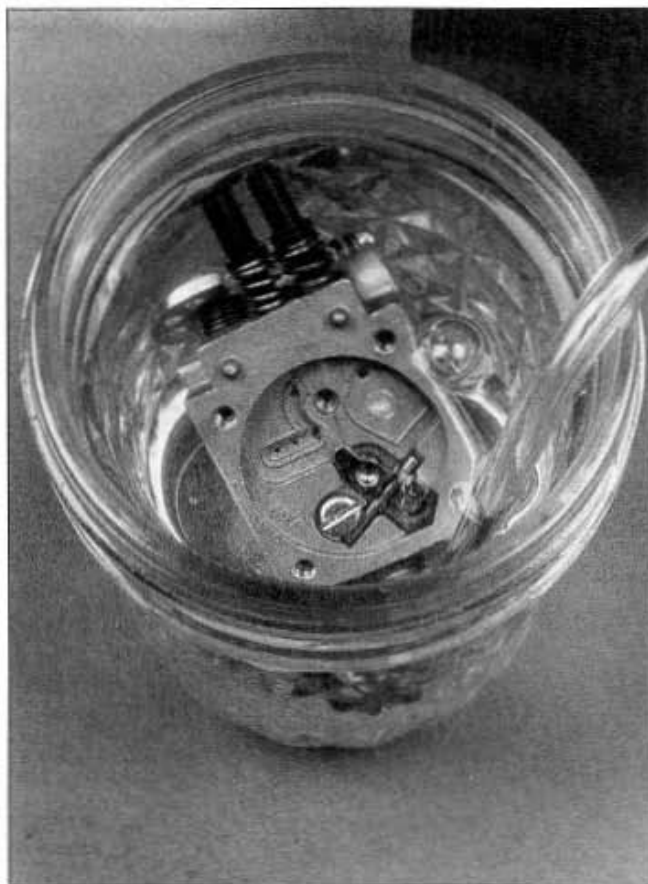
Bubbles from under the inlet needle, only after pop-off.
